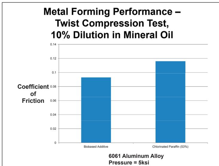
Figure 8 | A fluid formulated with 10 percent of a biobased boundary lubricity additive displays a superior coefficient of friction than a fluid formulated with 10 percent chlorinated paraffin in the Twist Compression Test run on a common aluminum alloy. (Courtesy of Croda Inc.)
