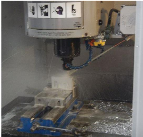
Figure 3 | A metal-removal operations involving an aluminum alloy is shown. (Courtesy of Machining Efficiencies Inc.)
