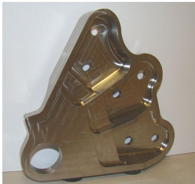
Figure 2 | The finished titanium-based roller cam plate is used in aircraft applications. (Courtesy of The Boeing Co.)
