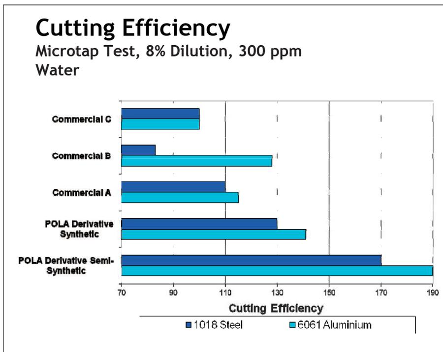
Figure 6 | Microtap test data shows that a POLA derivative can improve the performance of both a semisynthetic and synthetic fluid on aluminum and steel alloys. (Courtesy of Croda Inc.)
