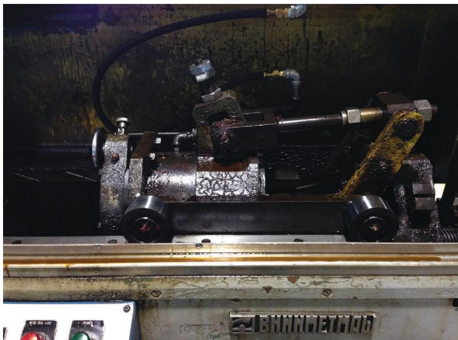
Figure 5 | An early 1970s tube roller designed by The Russian Institute and Design Institute of Metallurgical Engineering is commonly used to take over 70 percent overall reduction on zirconium, stainless and Inconel tubing. (Courtesy of Superior Tube Co.)
