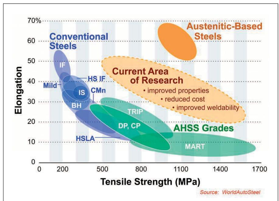
Figure 4 | The characteristics of the major steel alloys are shown in this graph of elongation versus tensile strength. Research is currently underway to develop new steel alloys in the section highlighted in light orange in this graph. (Courtesy of WorldAutoSteel.Org)
